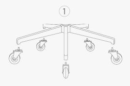
Install the rollers (11) into the crossbeam, as far as they will go.
