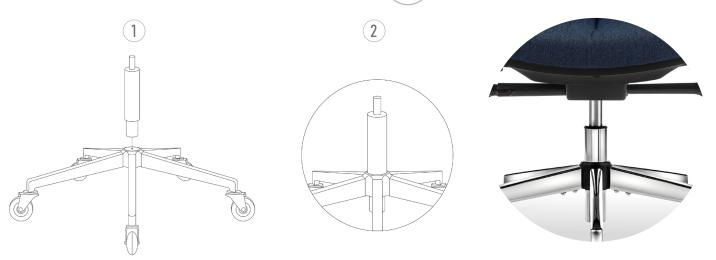
Place the gas elevator (5) into the hole in the crossmember.
